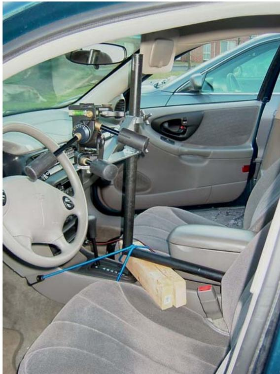
**Figure 34. Bracket for Radiant Imaging CCD Photometer.**
